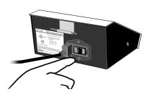
The voltage setting is designated at the factory before shipping. If the voltage shown does not match your power outlet, you must change the voltage selector before plugging the instrument into the outlet. To change the voltage selector:
