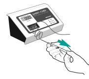
If desired, the specimen can be drawn back into the cell to repeat the measurement. If the plunger is moved smoothly and gently, the specimen can be transferred in and out of the conductivity cell for as many measurements as desired. Abrupt, jerky movements of the plunger can separate the liquid column, and the resulting air bubbles will interrupt readings as they pass through the cell.
