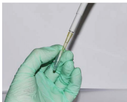
Figure 55 Pipette distilled water
