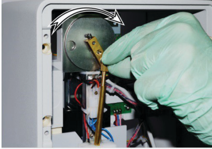
Figure 81 Check free movement of initiation needle
