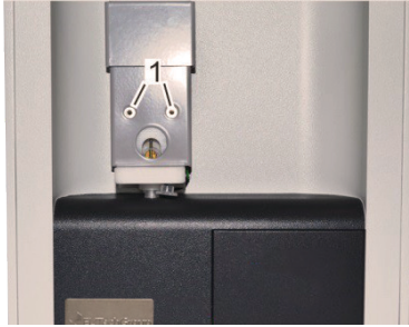
Figure 86 Remove mounting screws
