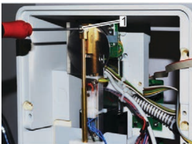
Figure 75 Remove mounting screw
