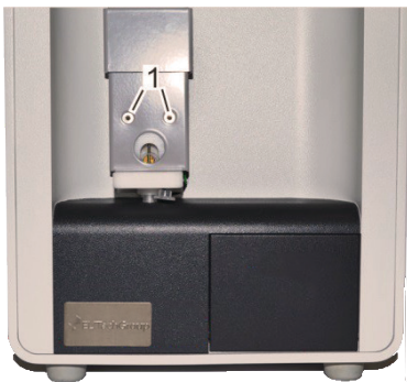
Figure 136 Tighten mounting screws
