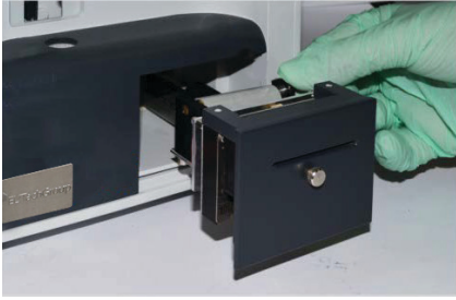
Figure 116 Turn knurled screw
