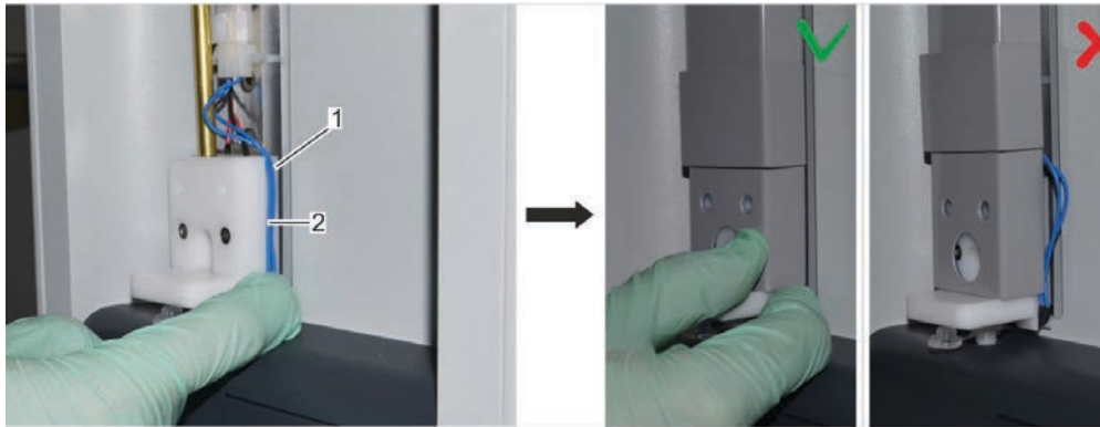
Figure 108 Elevator cover with correct cable routing
