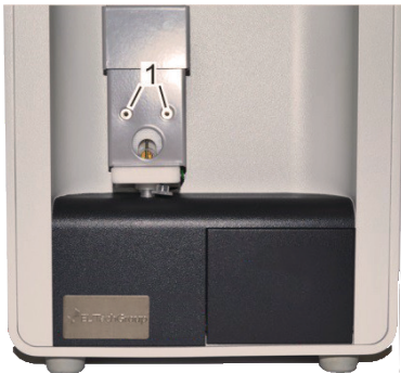
Figure 109 Tighten mounting screws
