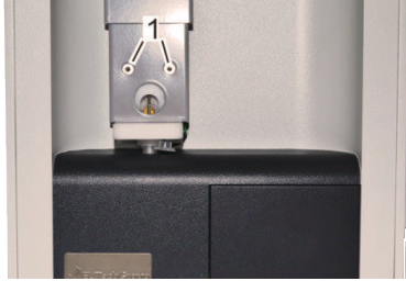
Figure 103 Remove mounting screws
