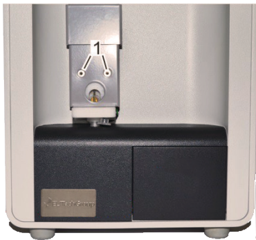
Figure 97 Tighten mounting screws
