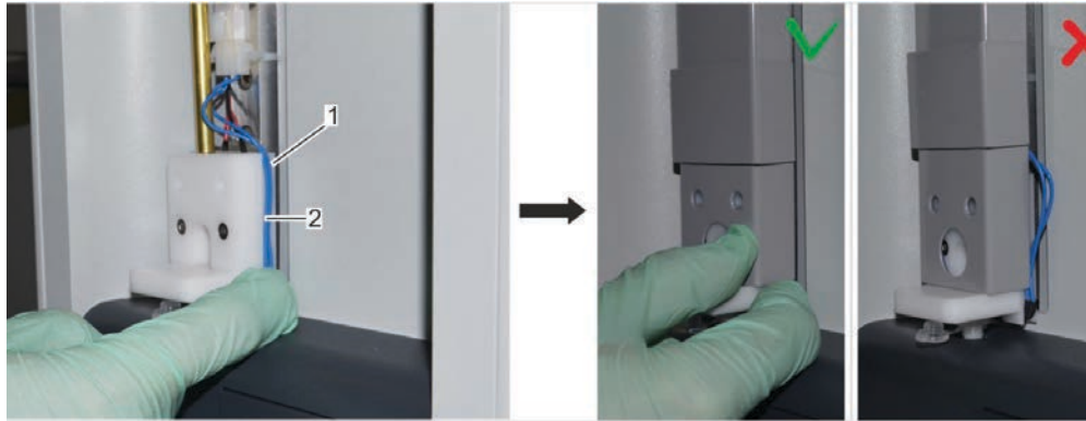
Figure 96 Elevator cover with correct cable routing
