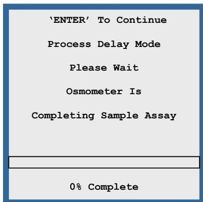
Complex samples (such as leaf and other semi-solid samples in nature from which water may not readily evaporate) require long periods to reach vapor equilibrium. Entering the *Process Delay Mode* allows the instrument to seal the sample chamber, but not to start the measurement process until the ENTER key is pressed. In research applications, this permits delaying the measurement until achieving vapor equilibrium.
