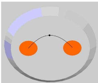
1. Place a waste container close by on the floor. Use a cotton swab to remove residue from the surface of the mount surrounding the thermocouple.
