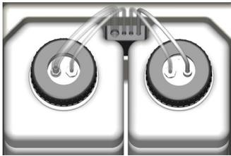
3. To install the supply reservoir, rinse, and then fill the reservoir with USP purified water. Place the filled supply reservoir in the instrument as shown (the waste and supply reservoirs are not interchangeable). Place the supply reservoir cap on the supply reservoir and tighten securely. **Make certain that the supply cap is used; do not cross the tubing and caps.**
