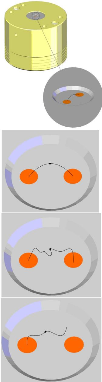
2. Carefully inspect the TC head under a microscope. Check for any gross contamination on the thermocouple or thermocouple mount.
