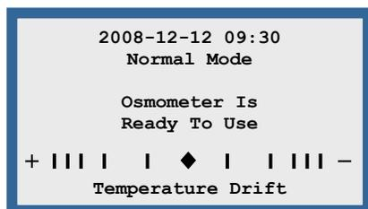
Osmolality determination involves the measurement of extremely small temperature differentials. The osmometer is thus sensitive to ambient temperature changes, which induce internal temperature changes.
