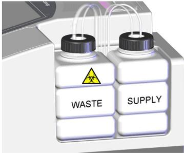
Note the location of the tubing in relation to the caps. Do not cross the tubing.
