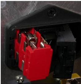
4. Replace both fuses with new fuses of the correct rating (5 x 20 mm time-delayed type 1A @ 250V).
