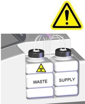
Note the location of the tubing in relation to the caps. Do not cross the tubing.
