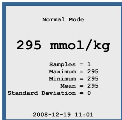
The progress bar along the bottom of the display shows the assay progress. When the measurement completes the tone sounds and the display screen shows the osmolality of the specimen. The display shows this final reading until the chamber closes again or another function is selected.
