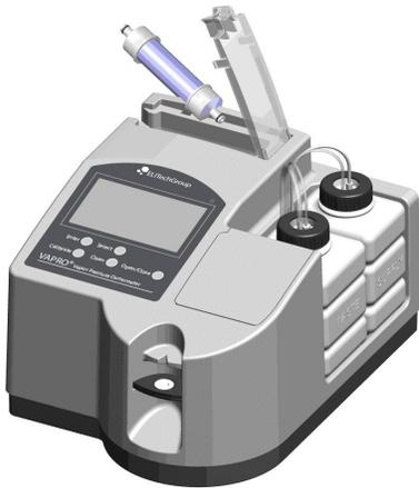
4. Remove the blue desiccant cartridge from the sealed bag. Remove the vinyl caps/plugs from the ends of the cartridge. Use the instructions in Section 4.3 to install the new cartridge.
