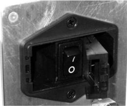
3. Pull the fuse holder out (you may need to use the small screw driver to pry it out).
