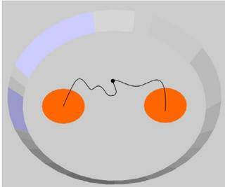
The thermocouple is well protected while the TC head is in the instrument. Cleaning procedures detailed in this manual should not harm the thermocouple; however, it can be deformed or broken if contacted by any object while it is out of the instrument.
