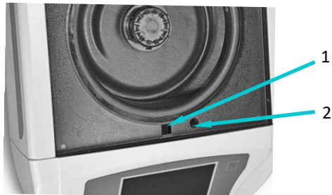
Figure 9: Lid Locking Mechanism and Pin Hole Locations
